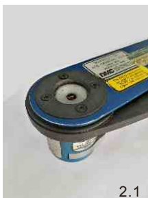
2.1 Adjust the locator of the crimp tool.
