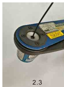
2.3 Insert the wire into the crimp tool, crimp the wire.
