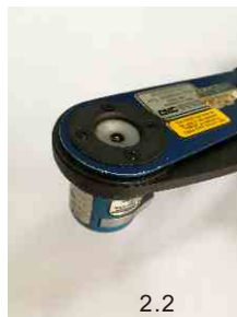
2.1 Adjust the locator of the crimp tool.
