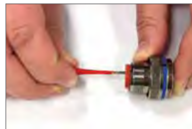
Plastic tool with contact in proper position.
