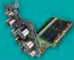
Press Fit Connectors on PC Board
