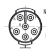
8MF1-PSM L: 85-264 VAC 4, 5, 6: Not connected
