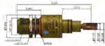
• LP-18-195-NF-X DC Pass N Type Female
