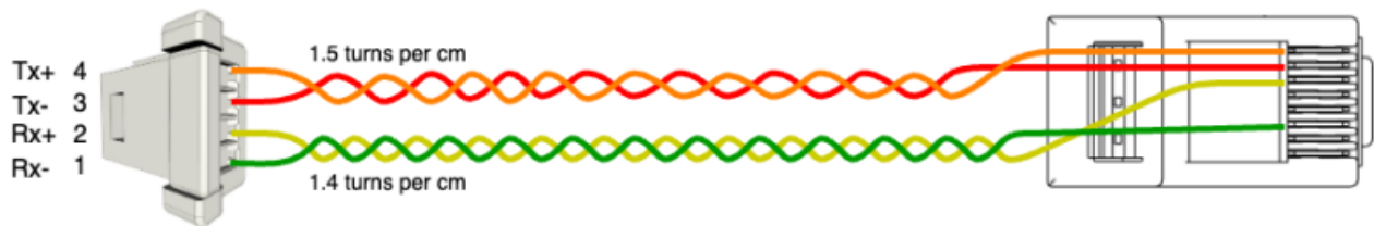
Ethernet cable pinout for Molex PicoClasp variant
