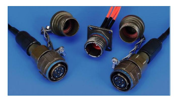
A high performance, harsh environment fibre optic connector. The MIL-C-38999 Series III connector can be specified as a dedicated fibre optic connector or a hybrid of fibre optics, power, signal, coax or data bus contacts.
