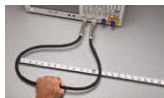
Flex Test (one full cycle)
