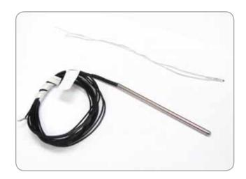
The Type CSP Temperature Standards are ultrastable probe thermistors which have been calibrated to an accuracy of 0.01°C. The standard unit has a thin, conformal coating of silicone rubber over the entire unit; this makes it suitable for immersion in a water bath. They are also available with stainless steel sensor housings, or they can be encapsulated into various sheaths. See assemblies depicted in the figure.
