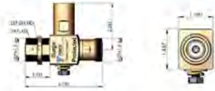
• LP-STR-DFF 800-2500MHz DC Blocked DIN Type F/F
