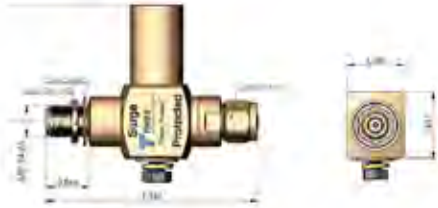
• LP-STR-NMP 800-2500MHz DC Blocked N Type M on Protected
