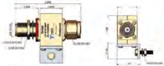
• LP-BTR-NMP 20-1000MHz DC Blocked N Type M on Protected
