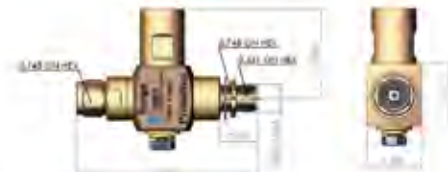
• LP-STRH-NMS 700-2700MHz DC Blocked N Type M on Surge
