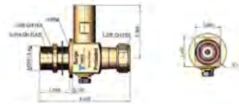
• LP-STRL-DMP 680-2200MHz DC Blocked DIN Type M on Protected
