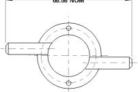
The Quick Calibration Hood is constructed from polypropylene, and provides a convenient means of supplying test gases to the VQ600 in the field, for calibration and checking purposes. The assembly push-fits into the central gas access recess of the head, and is designed to accommodate 6 mm ID or  $\frac{1}{4}$ " flexible tubing.
