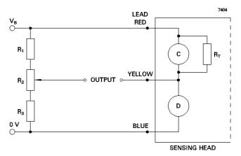
$R_1 = R_3 = 500$  to 5000  $\Omega$ ,  $R_2 \cong R_1/5$
