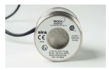
Although SGX Sensortech generally recommends that pellistors should be run with a constant voltage supply to the bridge, it is possible to use a constant current supply provided that the voltage across the bridge in clean air remains within the recommended limits.
