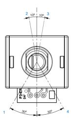
The detents are stops during the rotational travel that not only add a "click" sensation of position, but also offer enormous saving in both cost and space. PIHER's can feature special stepped outputs or 'constant voltage zones' for these detent positions and custom torques under request.
