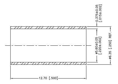
NOTE: ROCKWELL HARDNESS OF 65 MAX. ON 15-T SCALE
