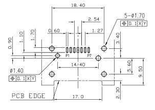
RECOMMAND PCB LAYOUT (GENERAL TOLERANCE: ±0, 05)
