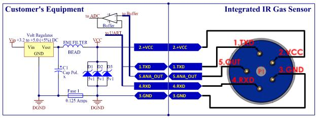
Fig. 1 -Example schematic for Interfacing Integrated IR (INIR)
