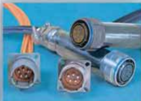
MIL-PRF-29504 Fiber Optic Termini can be accommodated in any size 16 or 20 contact cavity of MIL-DTL-38999 Series III connector.
