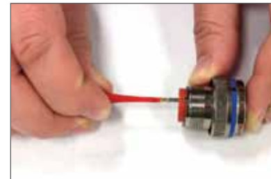
Plastic tool with contact in proper position.
