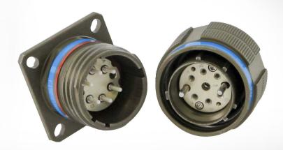
Based on the commercial ARINC 801 specification, this series features a removable alignment sleeve retainer (ASR) for ease of termini end-face cleaning, guide pins for precision alignment, and a scoop proof shell design.
