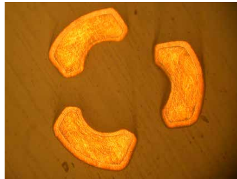
Au/Ni BARRIER (UNIFORM PLATING THICKNESS)
