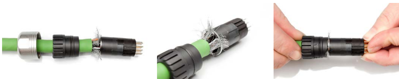
Step 10 - Position the shield as shown
