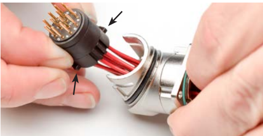
Step 5 - Locate keys on sides of insert
