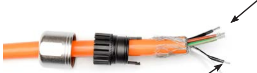
Step 5b - Strip signal wire 4.5mm
