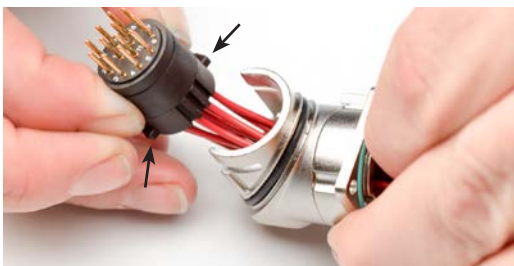
Step 5 - Locate keys on sides of insert
