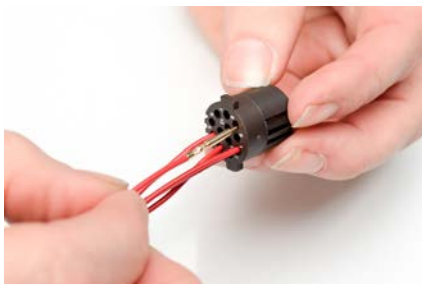
Step 4 - Push wire into insert
