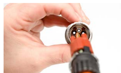
Step 14 - Trim shield as shown
