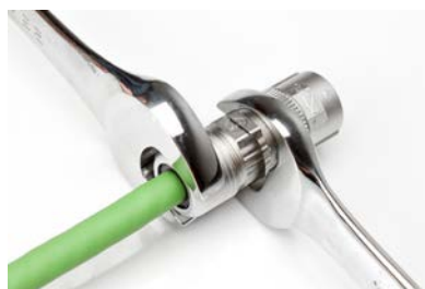
Step 16 - Tighten to 5-7 N/M using 25mm wrench
