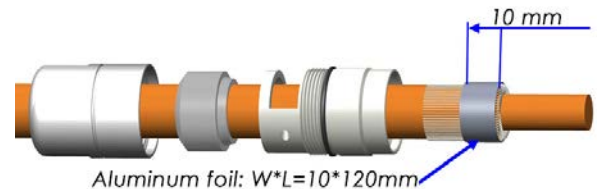
Step 4: Wrap foil over braided shielding
