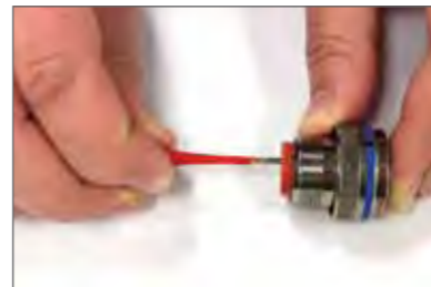
Plastic tool with contact in proper position.
