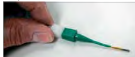
Plastic tool with contact in proper position.
