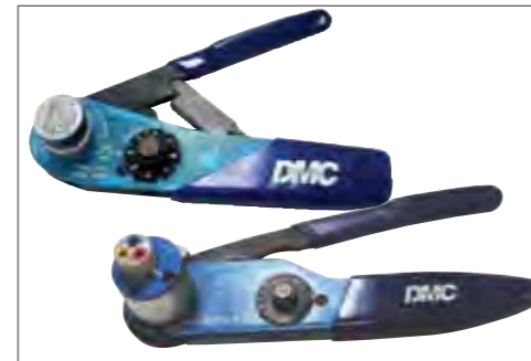
Examples of M22520 Series Crimping Tools: Shown top: tool used for small size 22, 22D and 22M contacts. Shown bottom: tool used for size 20, 16 or 12 contacts and has a positioner that can be dialed for each contact size.
