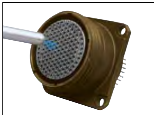
ESD Testing on MIL-DTL-38999, Series III Filter Cylindrical Connector (Actual Photo)
