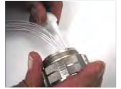
Use white end of plastic tool for removal of contacts.
