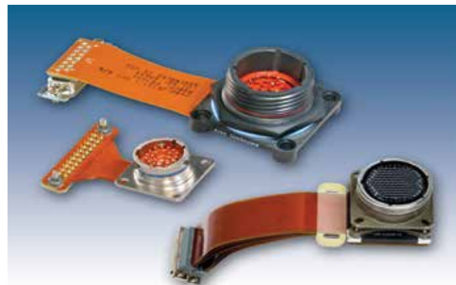
Flex Termination for Attachment to PC Boards
