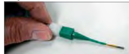
Plastic tool with contact in proper position.
