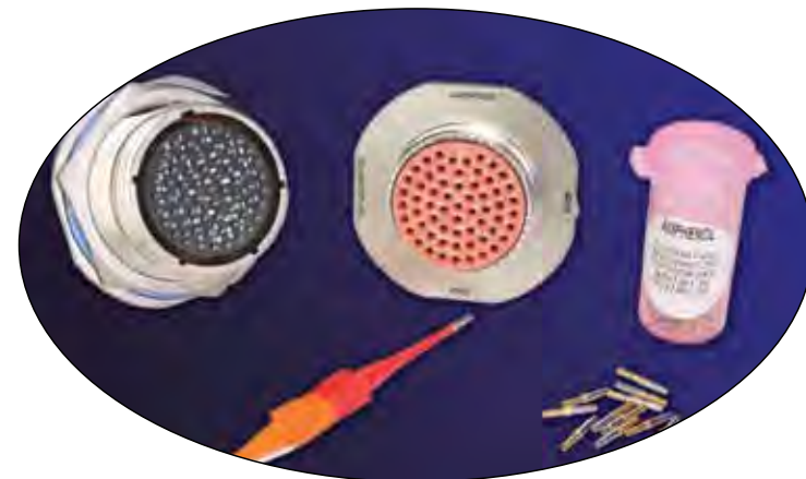
Sealed Jam Nut Receptacles (showing front and back) with Crimp Contacts - Use UTS Termination System with M39029/57 Socket Crimp Contacts and Standard Insertion/Removal Tool
