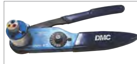
Example M22520 Series Crimping Tool for size 20, 16 or 12 contacts, and has a positioner that can be dialed for each contact size.
