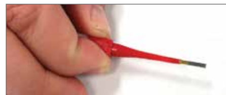
Plastic tool with contact in proper position.
