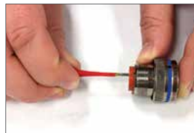
Plastic tool with contact in proper position.
