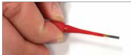
Plastic tool with contact in proper position.
