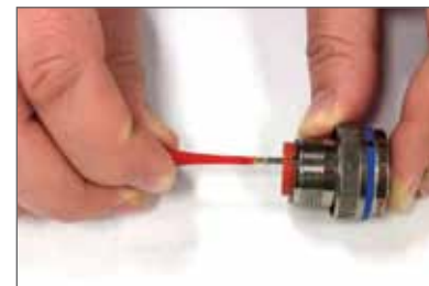
Plastic tool with contact in proper position.
