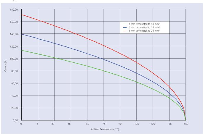
Remark: The given electrical values correspond to a single contact. With the addition of a housing, an increased number of poles or other modifications the values must be adjusted downwards accordingly
