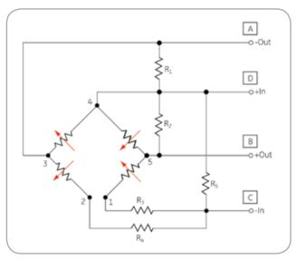
NPI-15 Series schematic diagram
