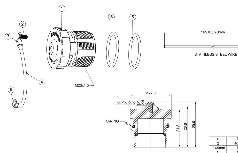
RRNBL14 **RING TERMIANL M4** 6  $\gtrsim$ RB000024 2 O-RING, 17.5MM(ID)\*1.6MM, BLACK VITON 5 165mm RM0061 STAINLESS STEEL WIRE 4 RSC000021 RING TERMIANL, M3 3 RM0084 RIVET,F2.5\*6.35 1 2 CP-M0837 METAL COUPLING NUT 1 DESCRIPTION ITEM QUANTITY PART NUMBER MATERIALS LIST
