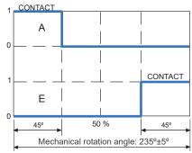
Power rating: 24V / 15mA ON position resistance:  $\leq 5\Omega$  Insulation resistance:  $\geq$  30M $\Omega$
