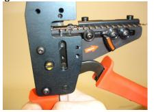
As shown on the picture, insert the strands of a stripped and straightened wire into the slot of the wire positioner. The insulation of the wire should be pouched to the surface of the wire positioner.
