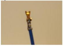
The tool is not cutting the carrier strip. In order to work properly, the operator has to cut the carrier strip on a regular base.
