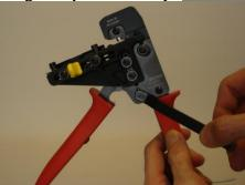
After the adjustment, install the locking screw again. Do never crimp without the locking screw in position.
