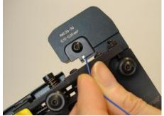
Whilst keeping carefully the wire in position, close the handles until the ratchet releases.
