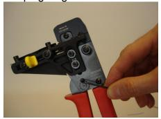
Be sure that the tool is open. Adjust the crimping height by means of the crimping height adjustment key. <u>Attention!</u> A miss adjusted crimping height can damage the tool.
