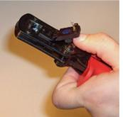
Push the locator towards the crimping die. A magnet will keep the locator in position.
