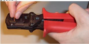
Release the levers and pull out the crimped contact.
