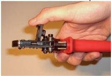
Introduce the contact. Push the contact till it reaches the hard stop.
