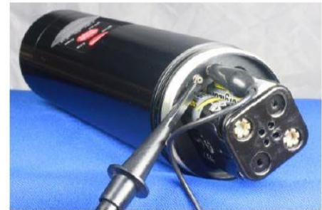
Figure 6: Probe connected to the test point pins
