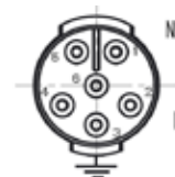
8MF1-PSM L: 85-264 VAC 4, 5, 6: Not connected
