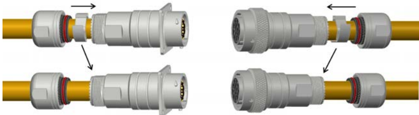
Step 11: Push shielding clip into backshell
