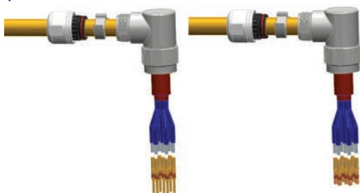
Step 7: Attach contacts to wire leads
