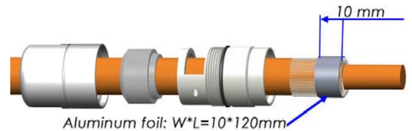
Step 4: Wrap foil over braided shielding
