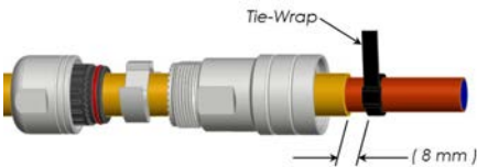
Step 3: Attach tie-wrap
