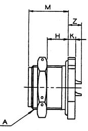
For contact data see Catalog 12-020. All lockwire holes .045 Dia. Min.
