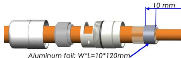
Step 4: Wrap foil over braided shielding
