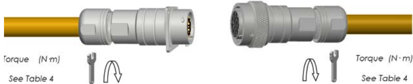
Step 13: Tighten metal nut
