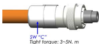
Step 9: Attach and tighten backshell as shown
