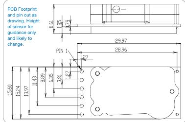
All dimensions in millimeters (mm)
