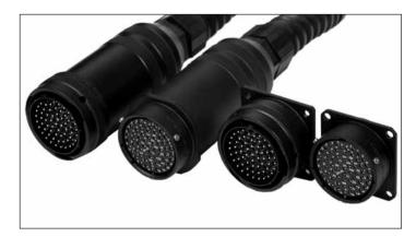
Amphenol's Multipin MP-62 series of circular connectors utilise the same design principles as the Mil-C-26482 military connectors. Featuring a three point quick mating bayonet coupling and five key polarisation ensuring a positive connection every time. Available in two contact pin layouts 39 and 61 with gold plated solder contacts fitted as standard.
