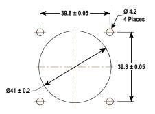
UPT07D-24-32P Size 24, 32 Way, Jam Nut Receptacle
