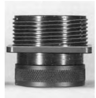
Standard double-lead Acme. Two parallel threads.
