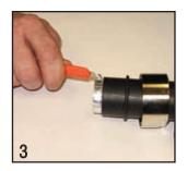
**Step 3:** Locate the inner drain wire (opposite the outer drain and under clear inner jacket). Slit the inner clear poly along the inner drain wire and pull back towards the jacket. Both drain wire will be exposed.
