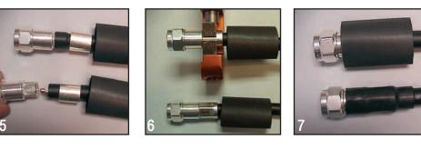
**Step 5**: Slide the connector over the end of the core and push it up to the end of the jacket. Rotate the connection back and forth in a clockwise-counter clockwise motion in reference to the axis of the cable until the back of the connector works its way under the end of the jacket. Now push the connector onto the cable with some back and forth motion until it stops.
