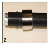
**Step 2:** Slide backnut and gasket onto cable. Trim and remove 13/32" of the cable jacket. NOTE: Do not cut the outer drain wire.
