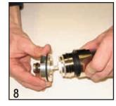
**Step 9:** Push in the connector inner conductor into the hollow copper tube inner cable conductor. Push on the connector head and attach to the backnut.
