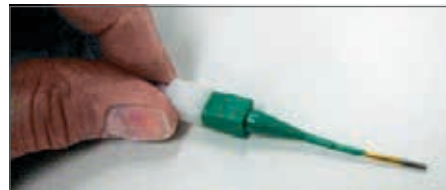
Plastic tool with contact in proper position.
