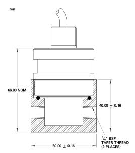
The Flow Cap allows the VQ600 to be used in applications where it is to be aspirated permanently with a pumped or pressurised sample. The cap is made of 316 stainless steel and can be used in a variety of applications involving pumped sampling analysis or detection systems.
