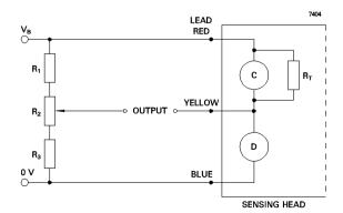
$R_1$  =  $R_3$  = 500 to 5000  $\Omega,~R_2 \cong R_1/5$
