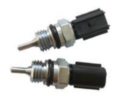
Thermometrics Coolant Temperature Sensor (CTS) monitors the temperature of the coolant that is being pumped around the battery to cool the battery module in Electric Vehicles (EV) and Plug-in Hybrid Electric Vehicles(PHEV). The purpose of this sensor is to relay signal to the battery management system (BMS) in the event of overheating. Should this happen, the vehicle can be stopped and the charging switched off before the heat causes any permanent damage to the battery
