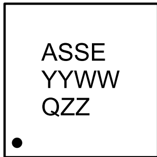
Figure 16. TDFN (3x3mm) 8-pin Marking
