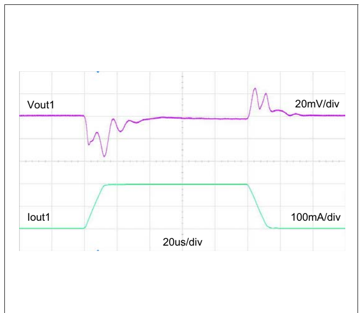
Figure 25: Load Transient Response Near Dropout, I_{OUT} = 200\text{mA}
