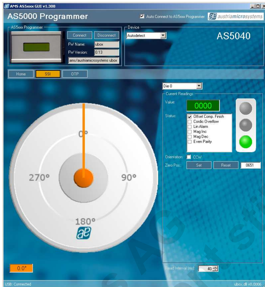
Figure 7: AS5040 SSI tab after Zero Position programming
